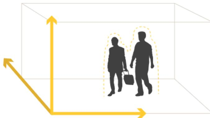
*Figure 1. A 3D solution uses information from its two sensors to evaluate depth in the image.*
