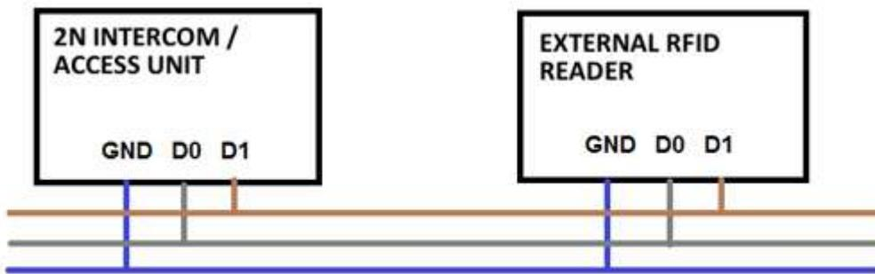
**Recommended Wiring Diagram for Reader with Bus Driver**
