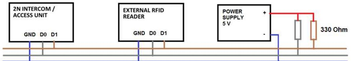
**Recommended Wiring Diagram for Reader with Open Collector (OC) Output**
