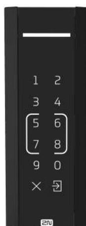
The white LED light indicates the power supply and operation states.
