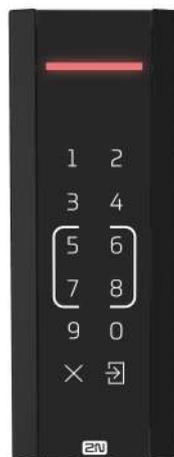
The red LED light goes on whenever an invalid PIN code is entered via the keypad or an invalid RFID card is applied. Subsequently, the set switch is not activated. An invalid authentication is indicated by an acoustic signal if set so.
