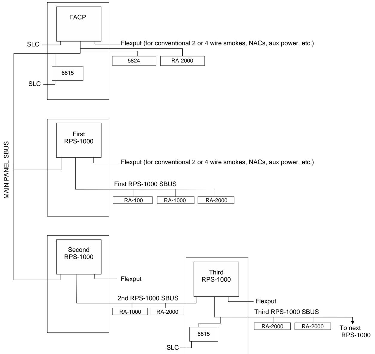
Figure 1.2 RPS-1000 Installation Overview (Details Added)
