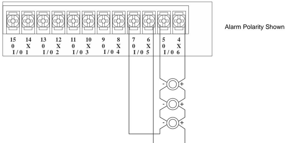
Figure 3.11 Class A Notification Appliance Circuit Configuration
