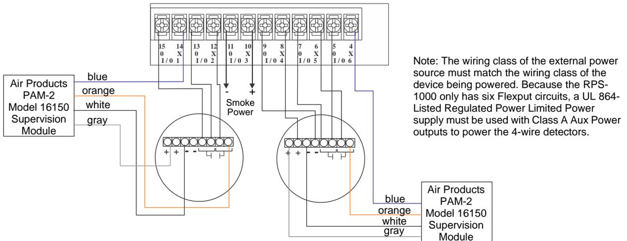
Figure 3.17 Class A 4-Wire Smoke Detector Connections
