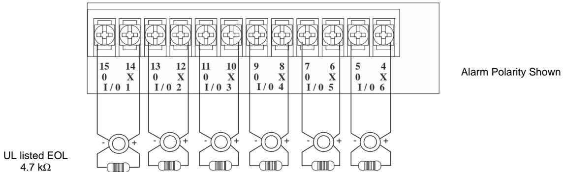
Figure 3.10 Class B Notification Appliance Circuit Wiring
