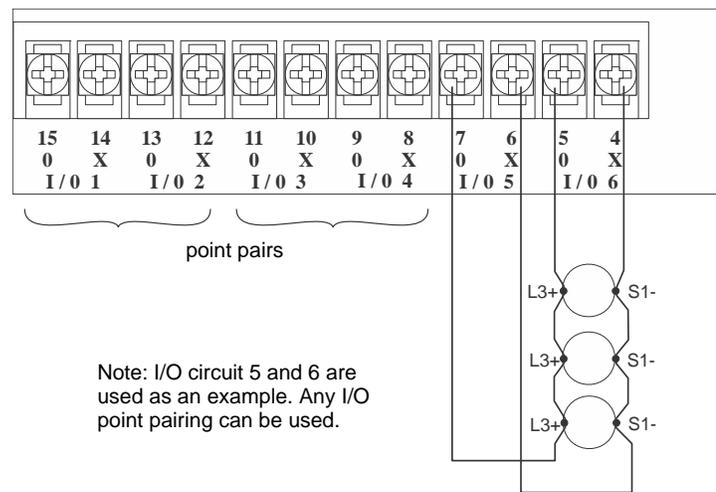
Figure 3.15 Two-Wire Class A Smoke Detector Connections
