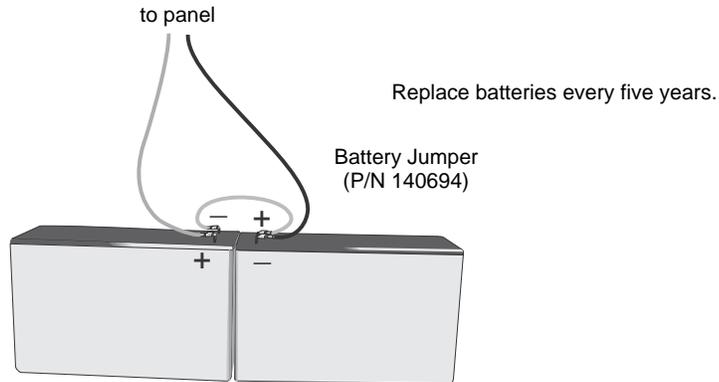
Figure 3.4 Battery Connection
