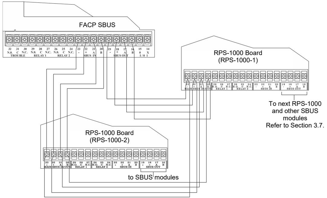
Figure 3.6 Class A RPS-1000 Connection to FACP
