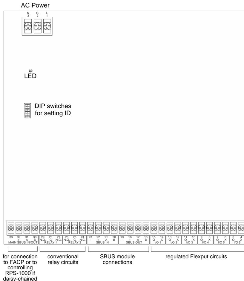
**Figure 2.1 RPS-1000 Board Layout**
