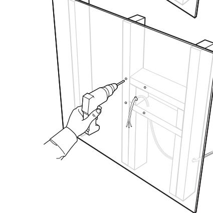
Minimum Installation Requirements when mounted to wood studs:  $\frac{1}{4}'' \times \frac{1}{2}''$  (M6 x 38 mm) lag screw
