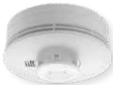
5800SMOKEV is a wireless photoelectric multi-criteria detector capable of detecting smoke, heat, rate-of-rise and low temperature. It is designed to provide early detection in the event of smoke and fire, and also reduces nuisance alarms from everyday cooking. The 5800SMOKEV has improved detection of smoke from common synthetic materials found in many modern home furnishings, which typically burn faster and hotter.
