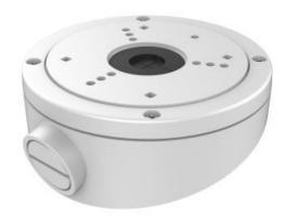
The bracket should be installed on a flat wall. Waterproof rubber is necessary for outdoor application. The wall must be capable of supporting over three times the total weight of the camera and mount. The maximum load capacity of the bracket is 9.92 lbs (4.5 kg).
