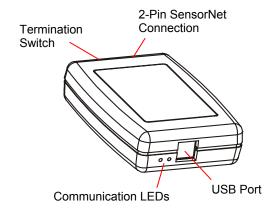
The USB Control Module allows a host computer, such as an Intellex digital video management system (or a PC with a USB port), to control one or more American Dynamics camera domes using the SensorNet (RS-485) communication protocol.
