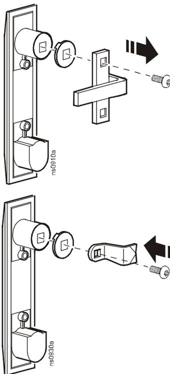
**To reverse the door handle:** If you reverse the door, complete the following steps to properly orient the door handle:
