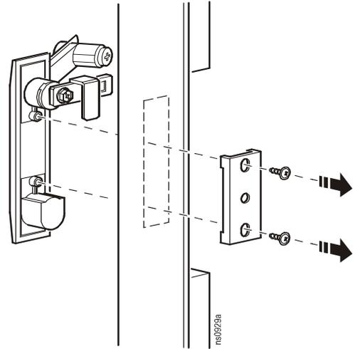
2. Remove the screw, cam, and washer from the back of the door handle assembly. Rotate the washer 90 degrees counterclockwise and the cam 180 degrees counterclockwise.
