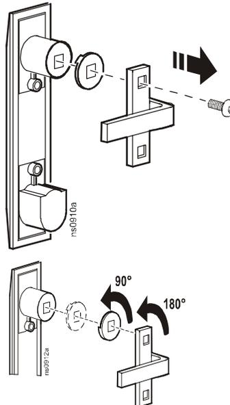
3. Re-attach the cam and washer.
