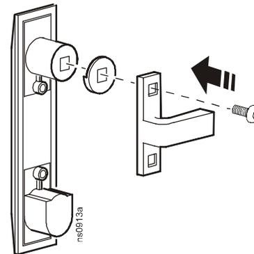
4. Reinstall the lock on the door as described in “To install the combination lock:” on page 2.
