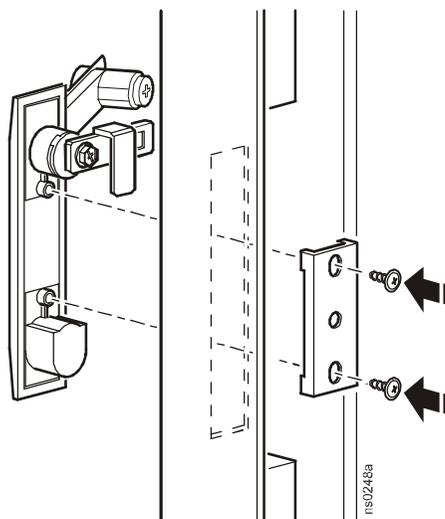
**To replace the cam:** If you have a NetShelter VX enclosure, replace the pre-installed NetShelter SX cam with the NetShelter VX cam (provided).
