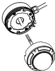
4. Route the cables through the cable hole (take side conduit cabling for example). Then reinstall the upper cover to the junction box.
