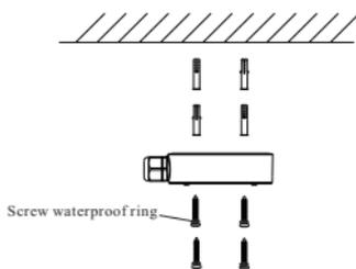
4. Fix the mounting base of the camera to the upper cover of the junction box. Then route the cables through the cable hole (take side conduit cabling for example) and connect the cables.
