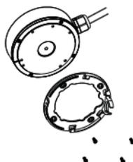
8. Remove the lower dome to adjust the view angle. After that, reinstall the lower dome to complete the installation.
