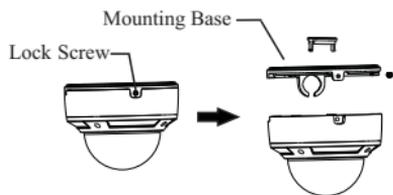
7. Connect the cables and then fix the lower dome to the mounting base by tightening the lock screw.
