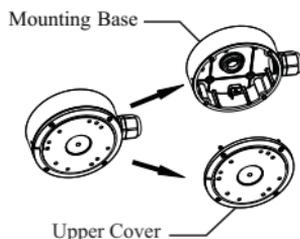
3. Push the expansion screws into the screw holes (if the wall is wooden, please skip this step) and then fix the mounting base of the junction box to the wall with screws.
