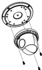
5. Route the cables through the cable hole (take side conduit cabling for example) and connect the cables. Then reinstall the upper cover to the junction box.
