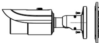
3. Fix the lower cover of the junction box to the corner mount with the nuts and bolts.
