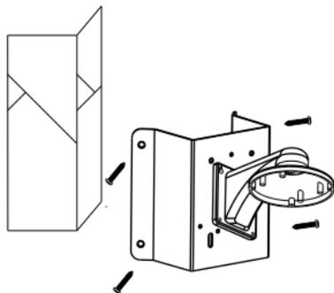
4. Screw the mounting base of the dome camera to the wall mount with screws.
