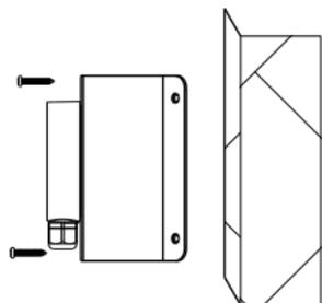
5. Tighten the covers of the junction box with screws.
