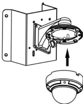
6. Fix the camera with lock screw.
