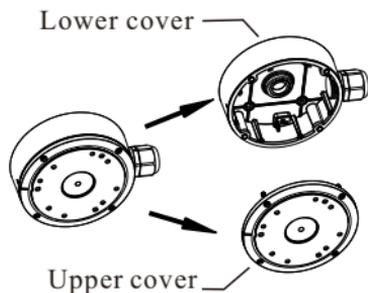
2. Screw the camera to the upper cover of the junction box.
