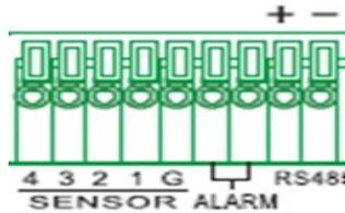
**Figure 4.4.3. Sensor, Alarm & RS-485 Ports**
