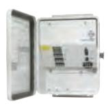
These power supplies provide 24 V AC output for one to four cameras. To compensate for voltage losses over long wire runs, 28 V AC outputs also are available on the WCS4-20. The power supplies have a selectable input of 120 or 230 V AC.
