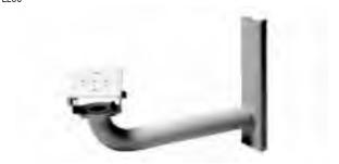
The EM1109/EM2000/EM2200 are medium-duty enclosure mounts designed for applications where mounting on a parapet or pole is necessary. These mounts can be used with Pelco enclosures having a 2-inch mounting hole pattern and are capable of supporting up to 40 lb. All three mounts feature a manually adjustable swivel head and a cable feed-through hole to conceal wiring. Multiple mounting holes on the tilt table provide 360 degree horizontal positioning of the enclosure.
