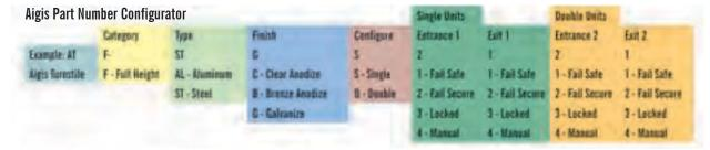
Example 1: (Single Unit) AT-FSTGS21 = A galvanized steel, single passageway turnstile with Fail-Secure entrance and Fail-Safe exit in the controlled direction(s). Example 2: (Double Unit) AT-FSTGD2121 = A galvanized steel, double passageway turnstile with Fail-Secure entrances and Fail-Safe exits in the controlled direction(s).
