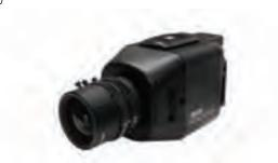
Smaller than most full-featured CCD cameras, the CC3751H-2 is ideal for use with one of Pelco's smaller enclosures (EH1000, EH3512, EH2512, EH2020, and EH2100). The CC3751H-2 has an extended Digital Slow Shutter (DSS) setting to enhance the low-light performance of the camera. DSS settings slow the picture frame rate and
