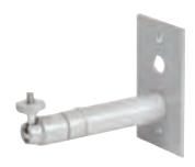
The C10-UM is a universal camera mount kit that includes all the components for wall, ceiling, or T-rail clip installations for most box type cameras with 1/4 x 20-inch mounting holes. The kit supports cameras weighing up to 7 lb (3.18 kg). The ball socket of the kit allows for 360-degree pan adjustment and 90-degree tilt adjustment.
