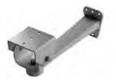
The EM1450 is a light-duty wall mount designed specifically for use with Pelco's EH3500 Series enclosures. Manufactured from die-cast aluminum, the EM1450 is capable of supporting a maximum load of 20 lb. (9 kg) and can be safely mounted to any vertical load-bearing surface.
