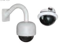
The D5 Series domes offer the ideal combination of high-quality, versatility, and cost competitiveness. High-resolution, 540 TVL cameras are available with a Sony CCD chipset for superb color performance, or a Pixim DPS Wide Dynamic Range imager for installations with bright light issues, such as bank lobbies and retail store fronts.
