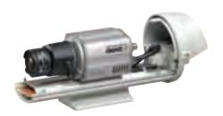
PixelPro iPak Kits include a housing and wall bracket with a preassembled Ganz PixelPro CS mount camera and Computar lens. Five feet of prewired outdoor rated power and Ethernet cables are included. IP65 rated aluminum housing.
