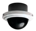
The IS150 Series Camclosure Integrated Camera System combines a camera and lens package into a small, high-security enclosure for medium-security installations subject to vandalism. The in-ceiling dome is designed for suspended ceiling or recessed ceiling/wall installations. An adapter plate is supplied with the dome to mount the unit to a 4S electrical box or to provide additional support for suspended ceiling installations.
