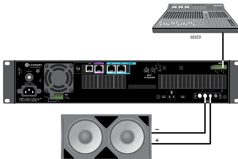
Figure 21 System Wiring Bridge Mode
