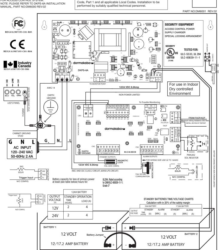
KEEP POWER LIMITED WIRING FROM NON POWER LIMITED WIRING AT LEAST 0.25" INCH APART
