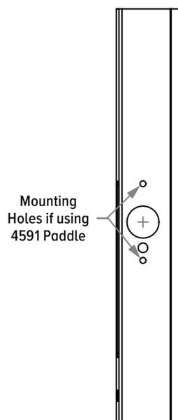
**DIAGRAM 5: Door Preparation: Lock Cut-Out to Backset/Cylinder**
