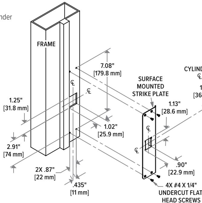
**DIAGRAM 2B: Door Preparation: Mounting holes for Reader\***
