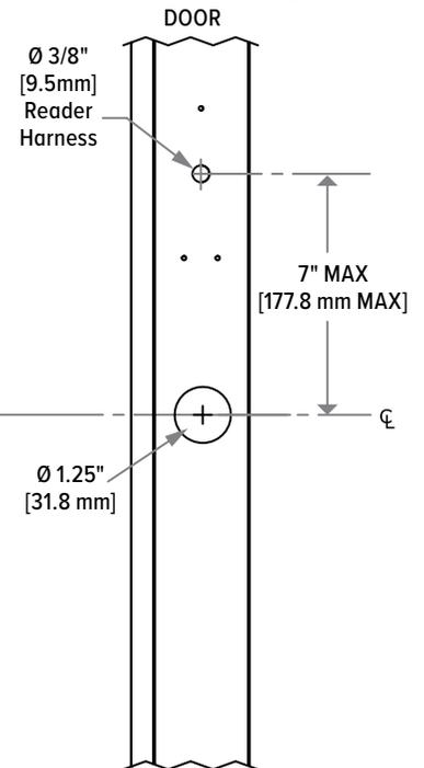
\*NOTE: Center Reader horizontally on Door Stile. Horizontal placement is Door Stile dependent.
