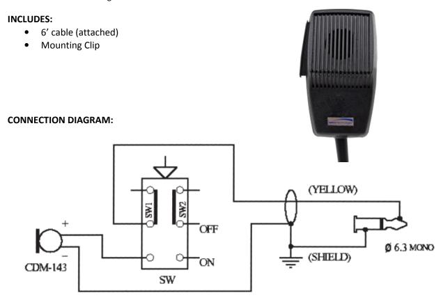
NOTE ON SWITCH TIMING: When Push to talk switch is pressed, SW2 contact closes before SW1 contact closes.
