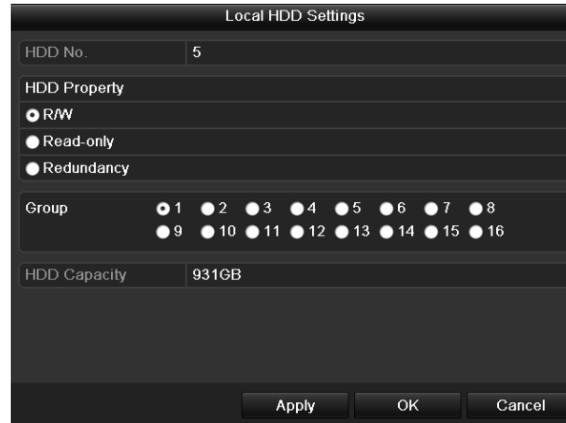
Figure 12-13 Local HDD Settings Interface
