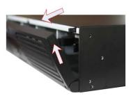
3. Inser the HDD bracket to the chassis along the slot unitl it has fully seated into position.
