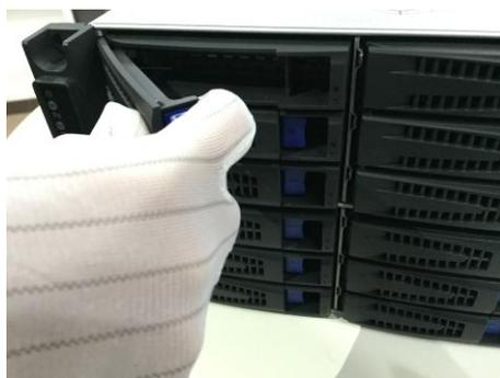
Figure 2. 3 Pull out the HDD Dummy
