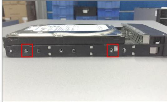
Figure 2. 5 HDD Position
