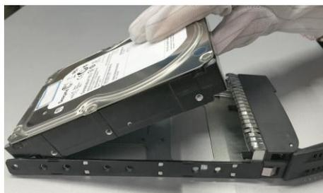
Figure 2. 4 Place HDD
