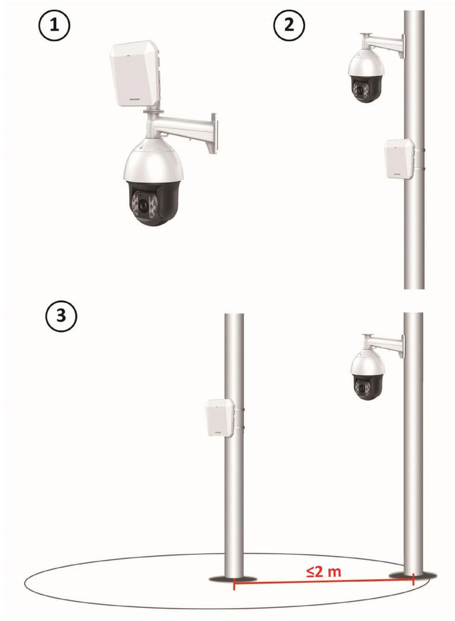
Figure 5-5 Installation Scene for One-Point Calibration
