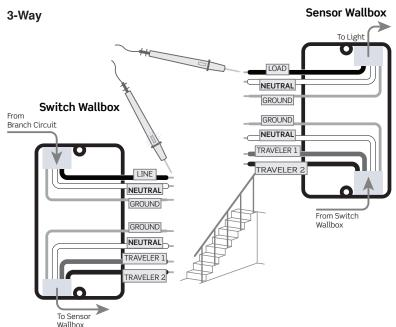
NOTE: Sensor must be installed in the location where the load wire is.
