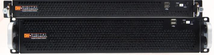
Blackjack® P-RACK™ servers powered by DW Spectrum® IPVMS support up to 128 2.1MP IP cameras with up to 600 Mbps throughput. Standard features include Intel® i7®, Windows 10® or Linux® Ubuntu® 16.04 OS on separate SSD, RAID and 2x NIC cards. Blackjack® P-RACK™ servers can be configured with 30-70TB HDD and come with our 5 year limited warranty.
