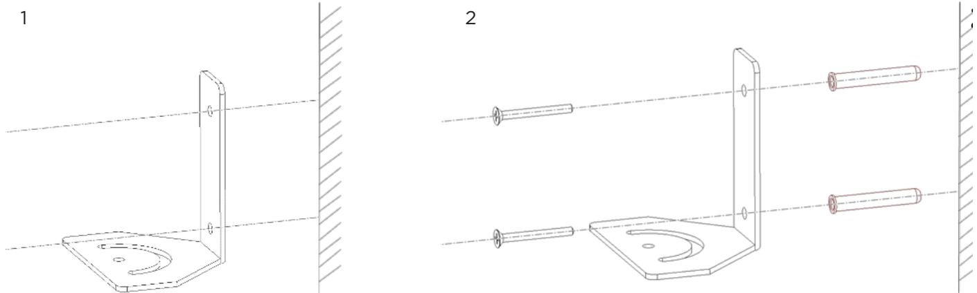
Use the bracket to mark and drill the necessary holes in the wall. \*NOTE: wall anchors are for illustration only, and are not included.
