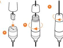
**NOTE:** To ensure moisture seal, make sure the o-ring is in place between a and In extreme environments use of an outdoor rated sealer is recommended.
