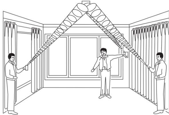
When the LED on the sensor goes solid momentarily while the tester is triggered, the glass is within detection range.
