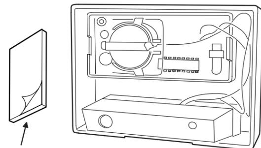
APPLY THE SUPPLIED DOUBLE STICK TAPE TO THE BACK OF THE TRANSMITTER AND SECURE IN CASE AS SHOWN
