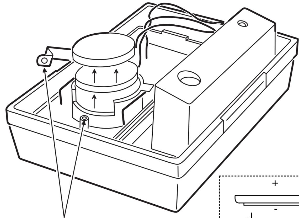
REMOVE BATTERY CLIP SCREW AND MOVE CLIP TO SIDE TO ACCESS BATTERIES
