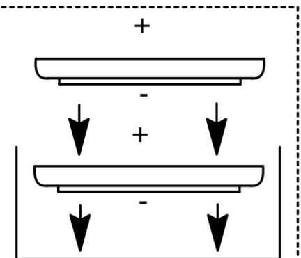
INSTALL TWO TYPE DL 2450 BATTERIES (+) SIDE UP
