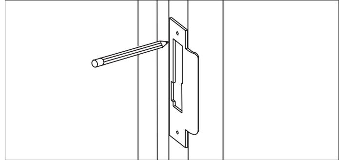
5. Remove material from within the strike outline so that the strike will be flush with the doorframe.
