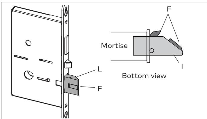
3. Using a small screwdriver, slide up the locking pin (P). Pull out the latch bolt (L) and rotate it 180°.
