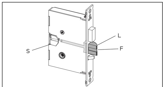
4. Pull out the latch bolt (L), until it just clears the front plate. (Note: If you remove the bolt completely, you must turn it 90° to re-insert it.)
