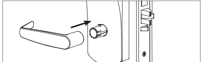
7. Three AA batteries should already be installed in the battery holder (C). Insert the battery holder into the outside housing and secure it using the 6-32 x 5/16" (7.9mm) Torx drive screw (H).
