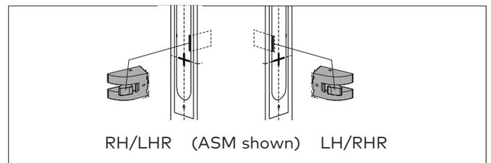
5. Drill the holes in the sides of the door (for dimensions, refer to template).
