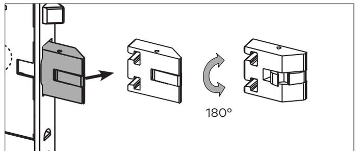
4. Re-insert the rotated latch bolt (L) until it stops. Push down pin (P) to lock the latch bolt in the mortise.
