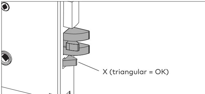
If the auxiliary latch (X) is a crescent shape, remove it, turn it 180°, and replace it. The auxiliary latch slides easily in and out of the mortise.
