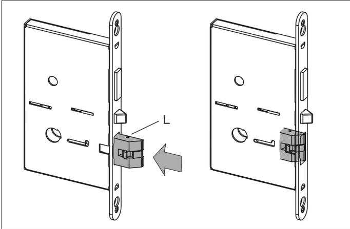
Release the latch bolt (L) while positioning anti-friction latch (F) so that it will remain inside the mortise. Ensure the bottom tooth of the anti-friction latch (F) remains inside the mortise case as shown.
