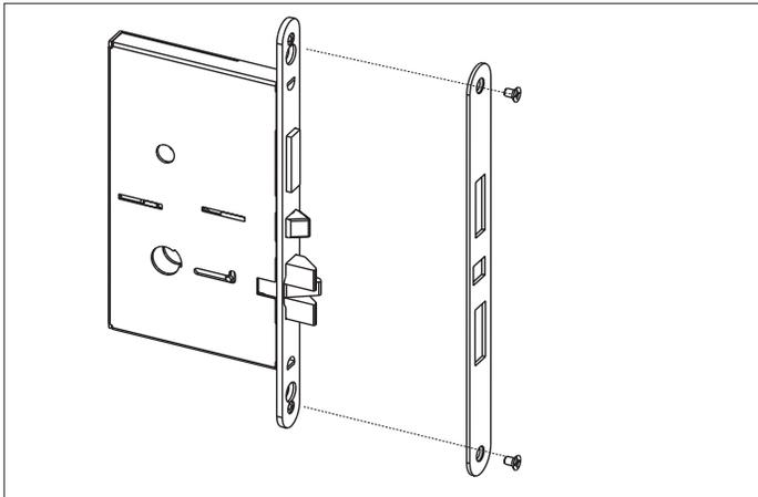
2. Retract deadbolt (D) as shown by turning the hub (H) with a small screwdriver, then push in the latch bolt (L) to the end of its stroke.
