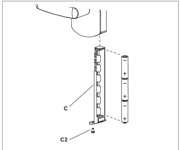
For E7900, after the mounting screws have been installed, insert batteries and refasten the battery enclosure cover into place.
