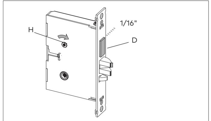
Hold deadbolt (D) gently. Press and release the auxiliary latch (X). You should feel the deadbolt trigger and begin to extend under the force of the spring.
