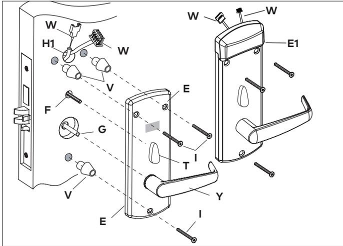
For 79T with ble or E, connect cables with corresponding connectors together (route the w6 in the switch holder as shown in the next figure) and put the excess cables in the area a when installing the inside trim.
