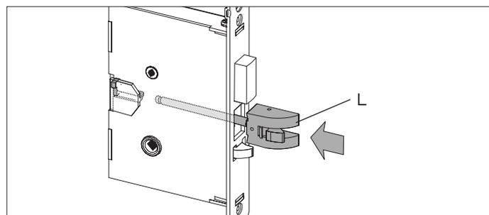
Holding tool (S) in place, re-engage tailpiece (T) with latch bolt (L) (slide tailpiece down). There may be some play required to align the parts. Remove the tool (S).
