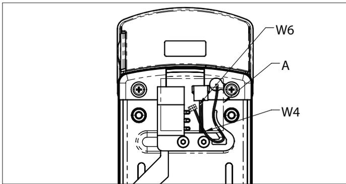
For E7900 series, the battery enclosure cover must be removed to install the mounting screws.
