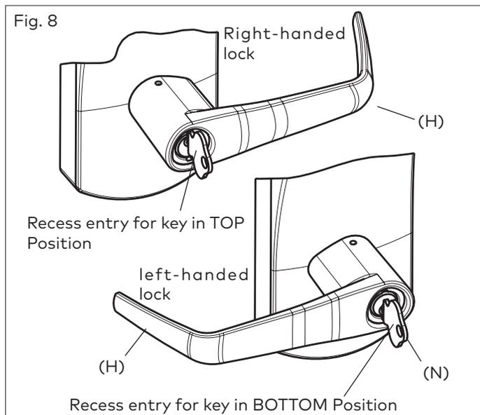
8. Press the lever (H) firmly against the housing while turning the key (N) counterclockwise (**this applies to both right-handed and left-handed locks**) until it is in the horizontal position. (Fig. 9)
