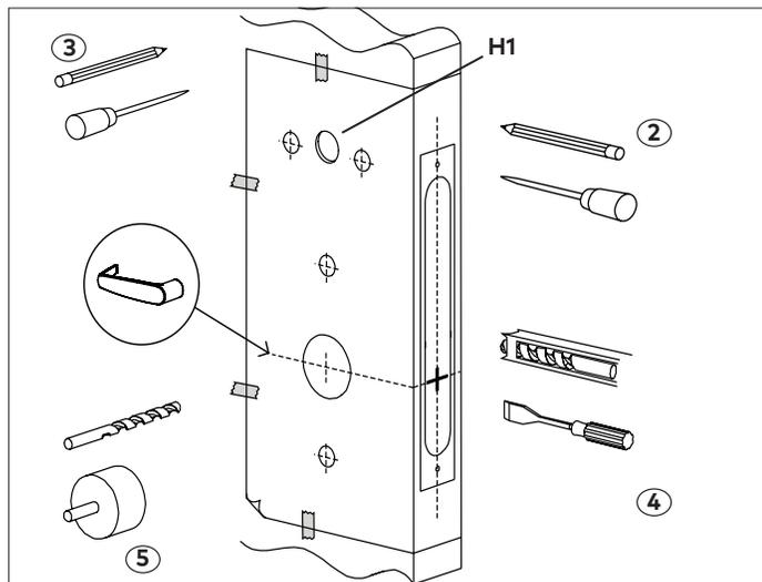
3. Locate the two sets of vertical fold lines on the template allowing you to adjust the positioning of the template depending on the bevel of the door.
