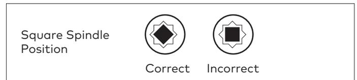
2. Insert the thumbturn spindle (F) in the upper hub of the outside housing. (It will clip in place.)
