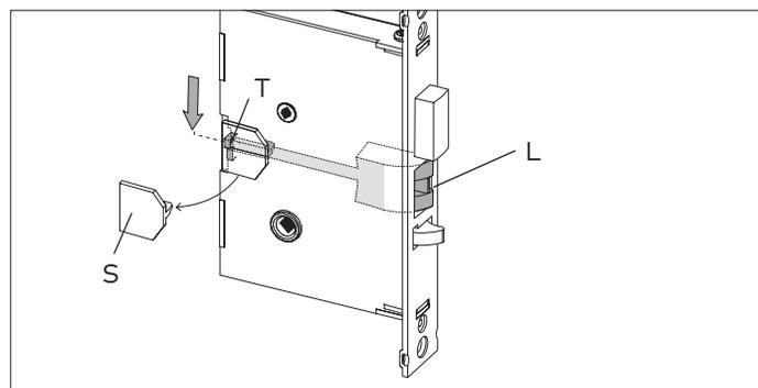
Release the latch to the middle of the stroke and hold it there. Use a small screwdriver to push the lock mechanism back on lock position (see step 1 and 2) .
