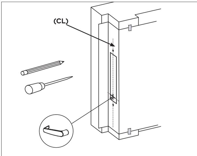
2. Mark the locations of the dust box cutout and mounting screws for the strike.
