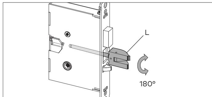
Rotate the latch bolt (L) 180°. Re-insert it to the end of its stroke.
