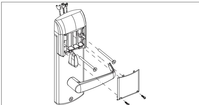
6. Assemble the lever on the outside housing, in the horizontal rest position appropriate to the handing of the door. Simply push the lever onto the tube until it clicks in place. If more force is required, use a rubber mallet. Test the attachment of the handle by pulling smartly on it. (For locks with mechanical override, see p.18)
