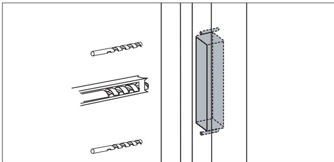
4. Position the strike against the doorframe and align it with the mounting screw holes. Trace the outline of the strike.
