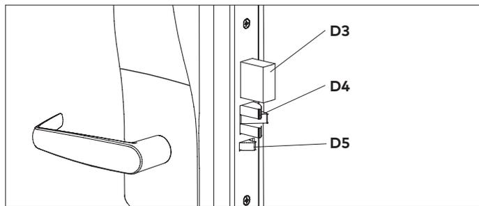
Release the auxiliary bolt (D5), then let the inside lever return to a horizontal position. The deadbolt will remain retracted while the latch will extend.
