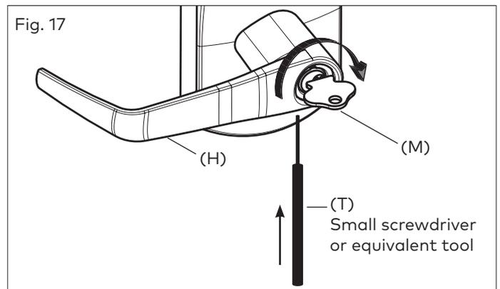
28. Pull the lever handle (H) off of the lock housing (be careful not to lose the cylinder plug (K) see page 18).
