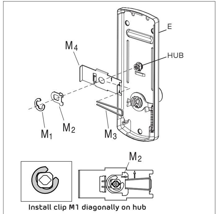
Turn the thumbturn all the way to the right for a RH installation (arrow on M2 points UP), or all the way to the left for a LH installation (arrow on M2 points DOWN). The thumbturn should stop in the vertical position, and the stopper cam (M2) will be in the position illustrated below.
