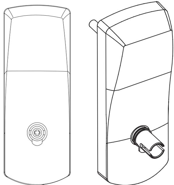
2. Preparing the outside housing for the installation of the lever handle
