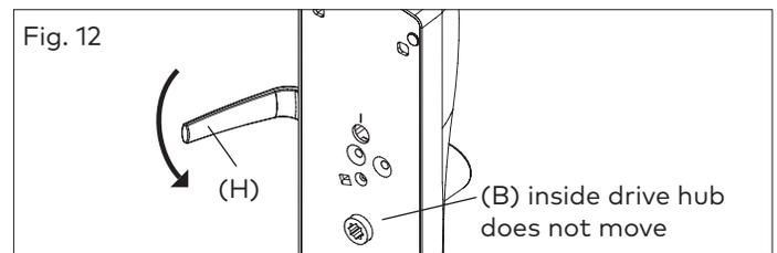
16. With the lever handle (H) in the horizontal position, insert the key (N) into the cylinder (J) and turn it clockwise **until it stops**. (This applies to both Right and Left-handed locks, see Fig.13)
