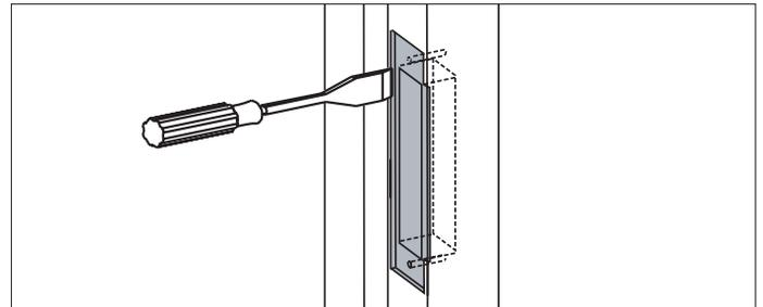
6. For ASM, install the dust box (optional for wood door frames, required for metal door frames), and check the strike handing on the template. Install the strike using the screws provided. Use wood screws for wood frame and mechined screws for steel frames.
