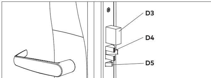
Release the auxiliary bolt (D5), then let the inside lever return to a horizontal position. The deadbolt will remain retracted while the latch will extend.
