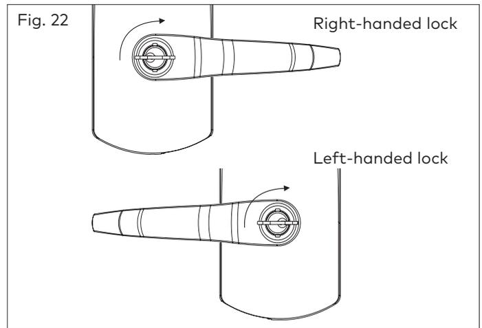
36. Turn the key back counter-clockwise until it is in the horizontal position.
