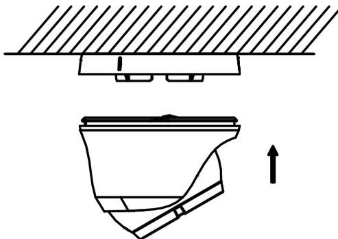
Figure 2-4 Secure the Camera with Mounting Base
