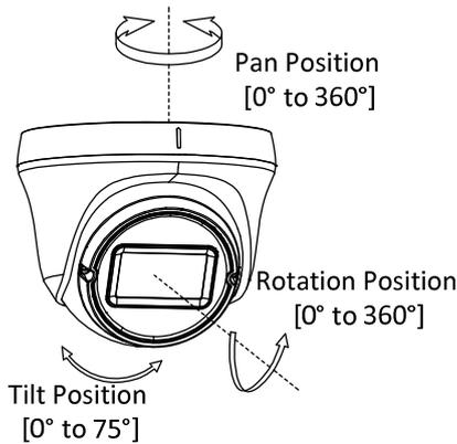
Figure 2-5 3-axis Adjustment
