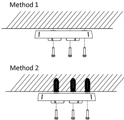
Figure 2-3 Attach the Mounting Base to the Ceiling
