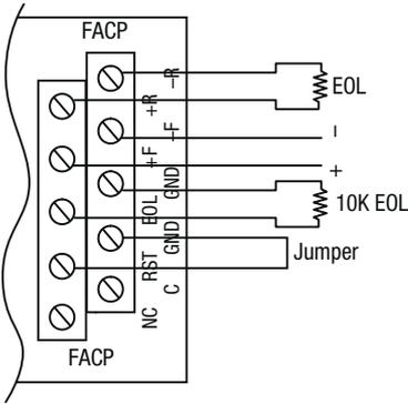
*Fig. 12 -* Polarity reversal input from FACP signaling circuit output (polarity is referenced in alarm condition).
