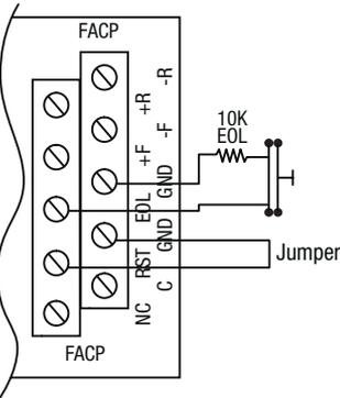
*Fig. 14 -* Normally Closed trigger input (Latching).
