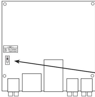
Fig. 2a - FACP Output - Dry Contact/Supervised Switch (Factory set to ON)
