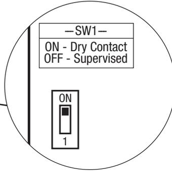
Fig. 3 - Entrada2DMT PC Board
