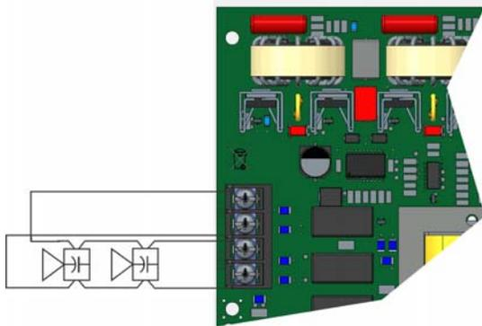
**Figure 7: Class A (Style Z) Speaker Configuration**
