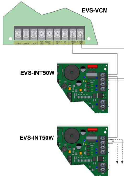
Figure 4: VBUS Wiring
