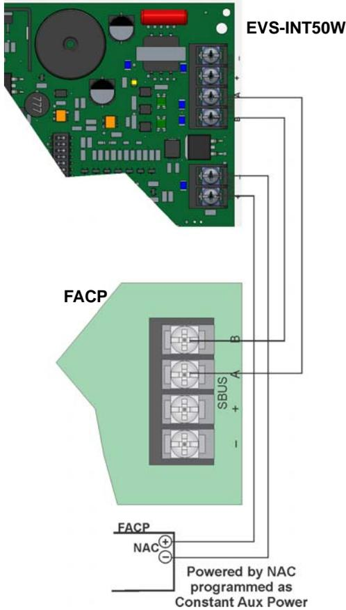
Figure 3: Wiring the EVS-INT50W to the FACP
