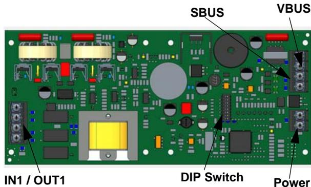
Figure 1: Front View of EVS-INT50W
