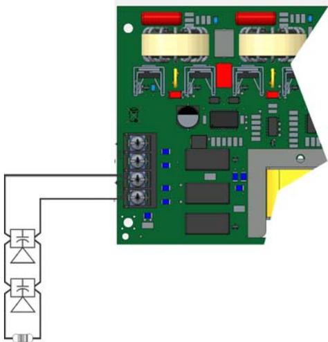
**Figure 6: Class B (Style Y) Speaker Configuration**
