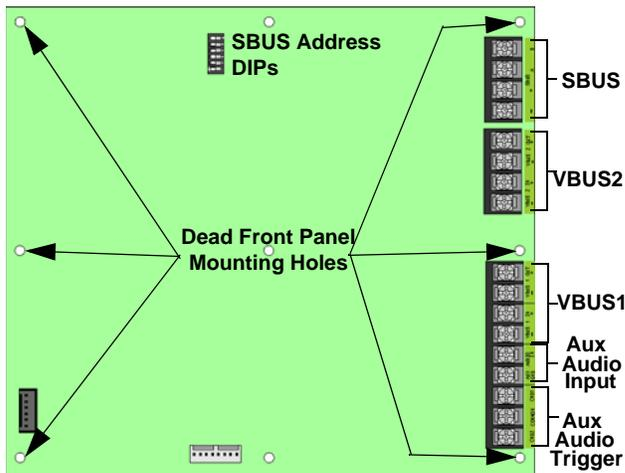
Figure 4: Back view of ECS-LOC board
