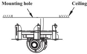
Route the cables through the ceiling and connect the cables. Then push the dome camera with the bracket into the mounting hole in the ceiling.
