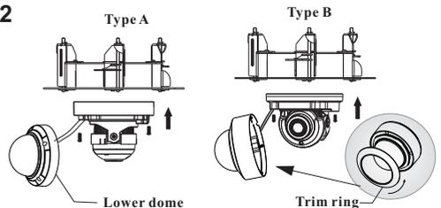
Remove the lower dome of the camera. Then place the in-ceiling bracket on the dome camera and tighten the screws provided to fix the bracket and the dome camera. (For type B, you shall rotate the trim ring anticlockwise to remove it. Then you can remove the lower dome by loosening the screws.)
