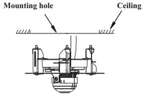
Route the cables through the ceiling and connect the cables. Then push the dome camera with the bracket into the mounting hole in the ceiling.
