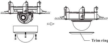
Install the lower dome back to the camera. Then put the trim ring onto the lower dome and rotate it clockwise until it is locked.
