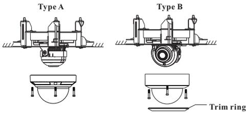
Install the lower dome back to the camera. (For type B, after installing back the lower dome, please put the trim ring onto the lower dome and rotate it clockwise until it is locked.)
