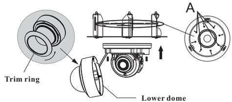
Rotate the trim ring anticlockwise to remove it. Then remove the lower dome of the camera by loosening the screws. After that, place the in-ceiling bracket on the dome camera and make sure the screw holes of the dome camera is aligned with the screw holes of the bracket marked with "A". Then fix the camera to the bracket with screws.
