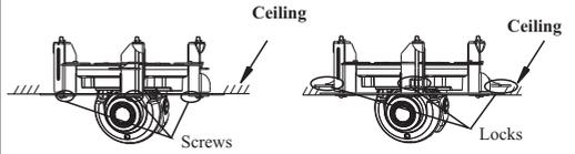
Tighten the lock screws with the screwdriver and the locks will automatically rotate outwards to secure the dome camera to the ceiling. Then adjust the view angle of the camera.
