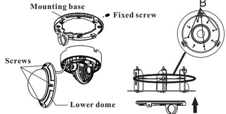
Loosen the screws to open the lower dome and then loosen the fixed screw to remove the mounting base. After that, make sure the screw holes of the mounting base are aligned with the screw holes of the bracket marked with "B" and then fix them with screws.
