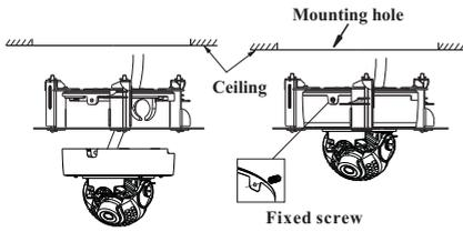
Route the cables through the ceiling and connect the cables. Then fasten the camera to the mounting base with the fixed screw. After that, push the dome camera with the bracket into the mounting hole in the ceiling.
