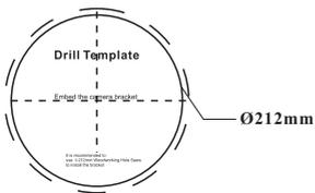
Attach the drill template to the ceiling where you want to install the dome camera. Then cut a hole according to the drill template. Note that +2mm of the circle diameter is allowed.
