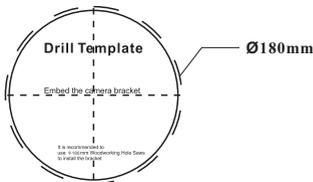
Attach the drill template to the ceiling where you want to install the dome camera. Then cut a hole according to the drill template. Note that +2mm of the circle diameter is allowed.
