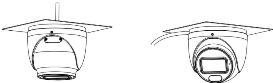
Then adjust the dome to obtain an optimum view angle.
