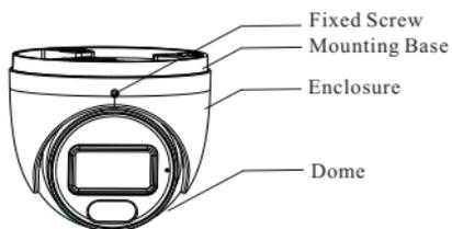
3. Secure the mounting base to the ceiling or wall with the screws provided.
