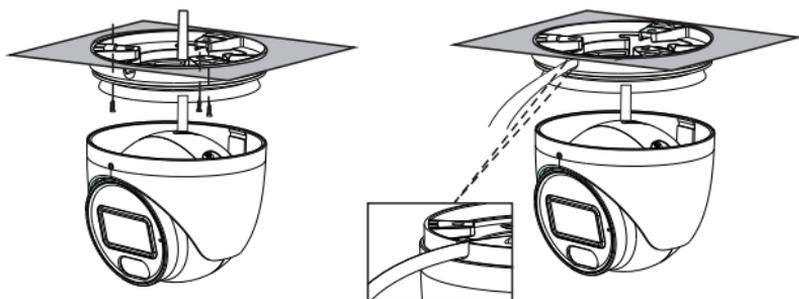
4. Install the dome and enclosure to the mounting base.
