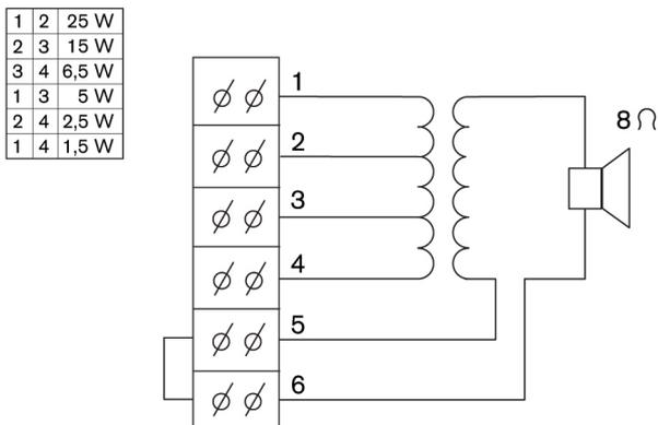
Fig. 2: Circuit diagram
