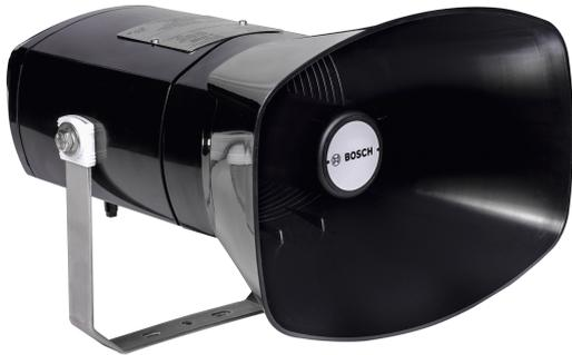
The LH3-UC25XL horn loudspeaker is specifically designed and certified for installations where explosive gas-air mixtures are likely to be present. The horn is constructed from anti-static Polyamid material, making the horn sturdy and light weighted. The longer flare design of the horn results in a higher sound pressure level where longer distance areas can be covered.
