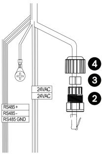
2. Slide one of each of the following pieces onto the RJ45 connector of the camera in sequence: end cap / nut (item 4), silicone seal (item 3), seal housing (item 2).
