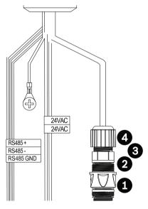
3. Connect the RJ45 connector of the camera to the RJ45 coupler (item 1). Connect item 2 to item 1. Slide item 3 into item 2. Connect item 4 to item 2.
