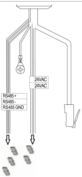
1. Remove the five (5) quick-connect connectors from the ends of the cables at the base of the camera.
