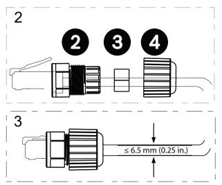
4. Repeat steps 2 and 3 for the Cat5e/Cat6e cable from the head-end IP network. **Note:** An RJ45 cable with a large sheath may not fit completely into the RJ45 coupler. Bosch recommends using a cable *without* sheathing.
