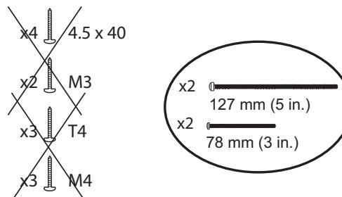
Note: When installing some FLEXIDOME cameras (such as NIN-70122-F0A), use the M4 washers to prevent the screw head from falling through the mounting hole.
