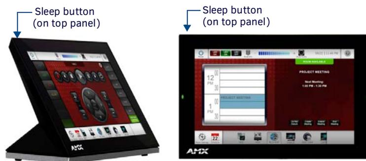
**FIG. 2** Sleep Button location - Tabletop and Wall Mount
