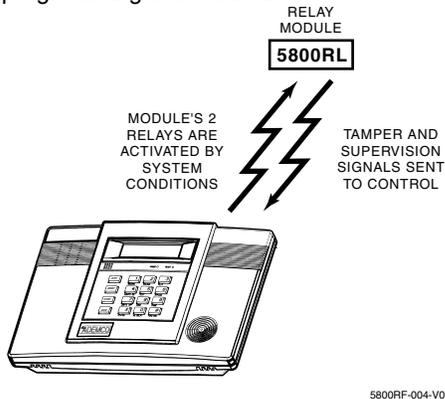
Figure 1. Lynx Interface Diagram
