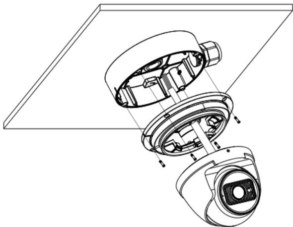
⑦ Adjust the camera to obtain an optimum angle. Before adjustment, preview the image of the camera on a monitor. After that, tighten the set screw to finish the installation.
