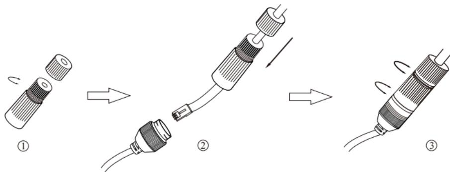
① Loosen the nut from the main element.
