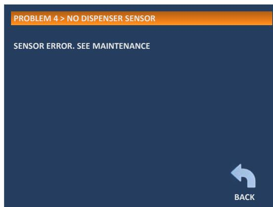
**POSSIBLE CAUSE:** A buildup of debris in the dispenser rotary caused by not cleaning the dispenser sensor often enough.
