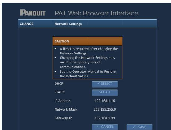
When the IP Address Mode is changed, an IP Address, an optional Network Subnet Mask and optional Gateway address can also be entered. The IP Address Mode can be restored to the factory default value as described in *Restore* section on Page 64.
