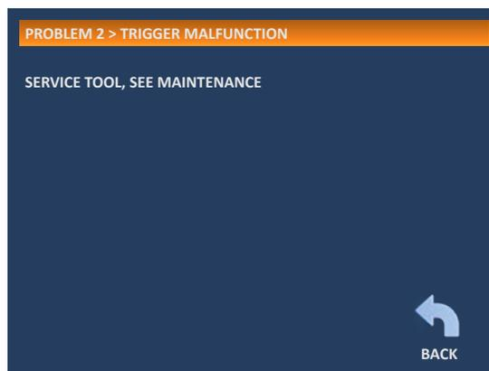
**POSSIBLE CAUSE:** This message will appear if the trigger is held down or stuck when the dispenser is turned "on". This message will also appear if the switch has malfunctioned.
