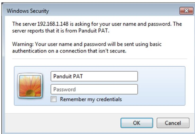
When first accessing the Network and Setting pages on the PAT SYSTEM; or after approximately 30 minutes of inactivity, entry of a Username and Password is required. The default Username is "Panduit PAT" and the default Password is "password".
