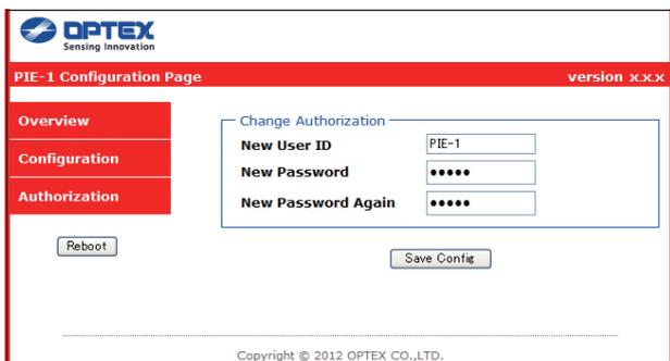
In the Authorization screen, you can change the user ID and password when accessing the web screen. After changing the settings, click the [Save Config] button at the bottom of the screen to save the settings in PIE-1.
