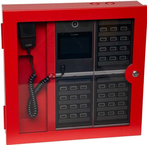
This first responder panel is a full function Local Operating Console (LOC) or Autonomous Control Unit (ACU) and is intended for the use in PRAESENSA mass notification systems. It has a red wall-mount enclosure with a key-locked transparent front door, and comes standard with one LCD call station (PRA-CSLW), and three call station extensions (PRA-CSE).
