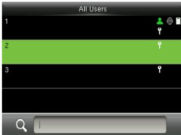
**Add a Normal User:** Choose “Normal User” in [**User Role**]. When the Super Admin is set, Normal Users can only use fingerprint, password or card for verification; when the Super Admin is not yet set, Normal Users can operate all functions on the menu.
