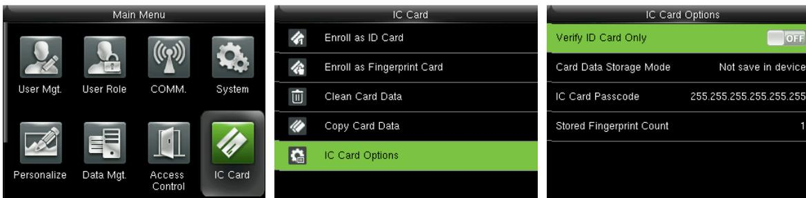
In the initial interface, press to enter the main menu, then press to select **IC Card** and press to enter
