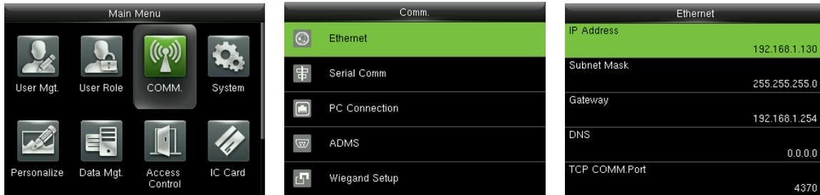
In the initial interface, press > **Comm.** > **Ethernet** to enter the **Ethernet** setting interface.
