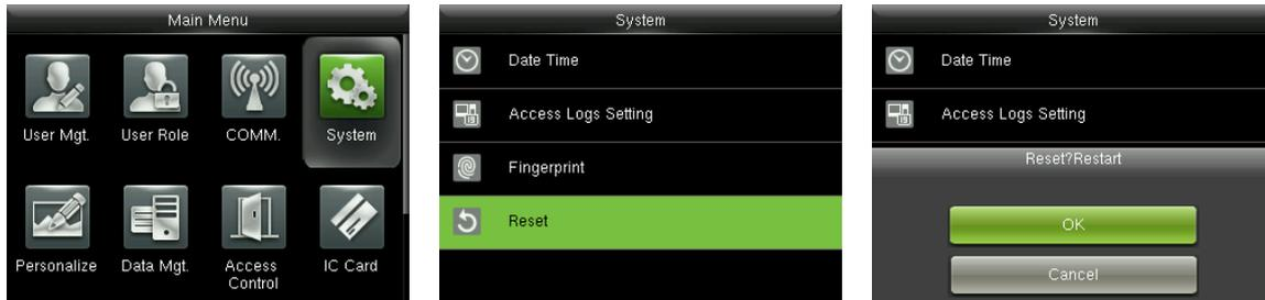
In the initial interface, press > **System** > **Reset** > **OK** to finish the reset setting.
