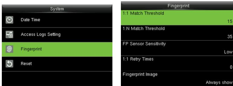
In the initial interface, press > **System** > **Fingerprint** to enter the **Fingerprint** setting interface.
