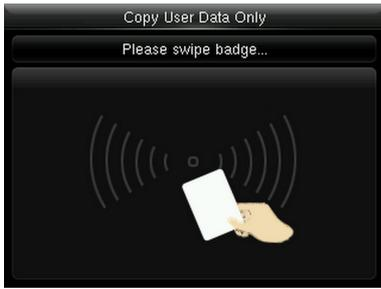
Put Mifare card in the card area, waiting for the device to copy user information (user data only or user data and fingerprint) to the device
