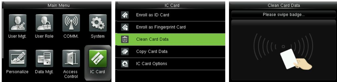
In the initial interface, press  $\rightarrow$  to enter the main menu, then press  $>$  to select **IC Card** and press  $\rightarrow$  to enter
