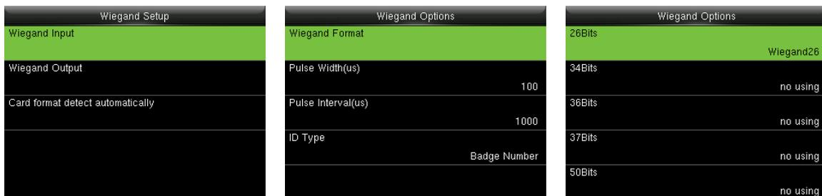
Select "Wiegand Input" and Set parameters in "Wiegand Input" interface
