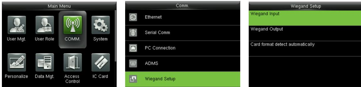
In the initial interface, press > **Comm.** > **Wiegand Setup** to enter the **Wiegand Setup** setting interface.
