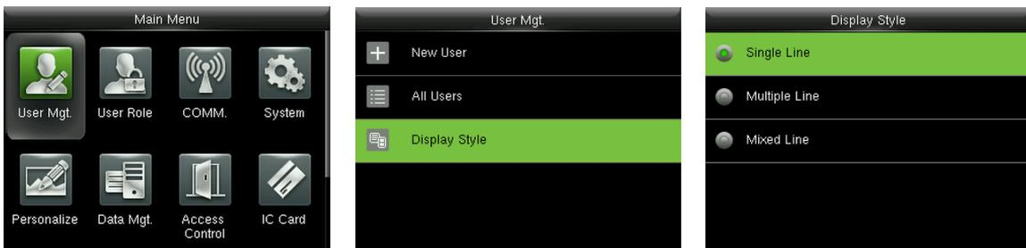
In the initial interface, press
