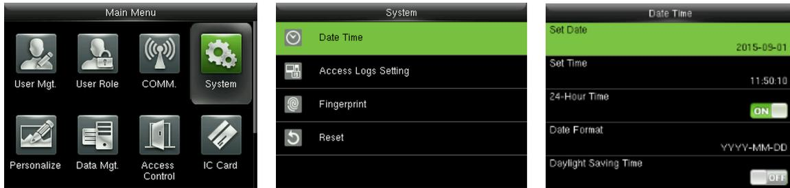
In the initial interface, press > **System** > **Date Time** to enter the date/time setting interface. It includes setting date, time, 24-hour clock, date format and daylight saving time.
