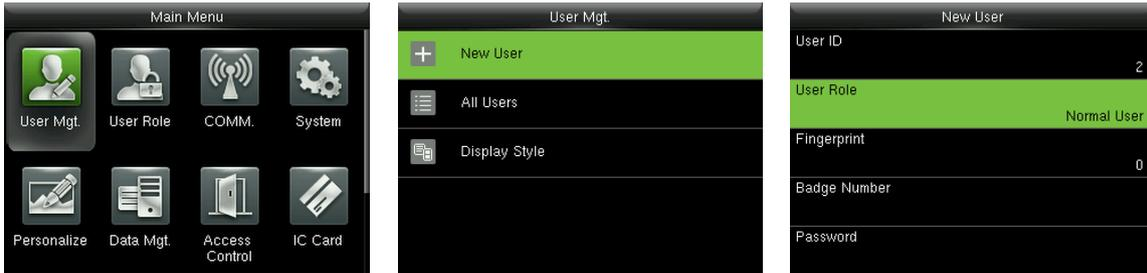
In the initial interface, press > **User Mgt.** > **New User** to enter **New User** setting interface. Settings include inputting User ID, choosing User Role (Normal User / Super Admin), registering Fingerprint and Badge Number, setting Password and setting Access Control Role.
