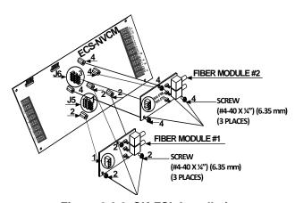
Figure 3.2.2 SK-FSL Installation
