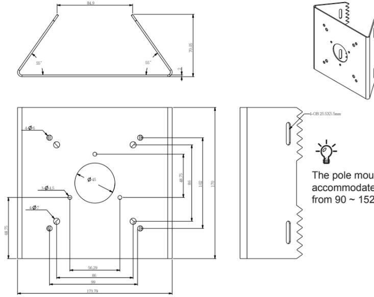
The pole mount bracket is designed to accommodate a pole in a diameter ranging from 90 ~ 152mm (3.5 ~ 6 inches)
