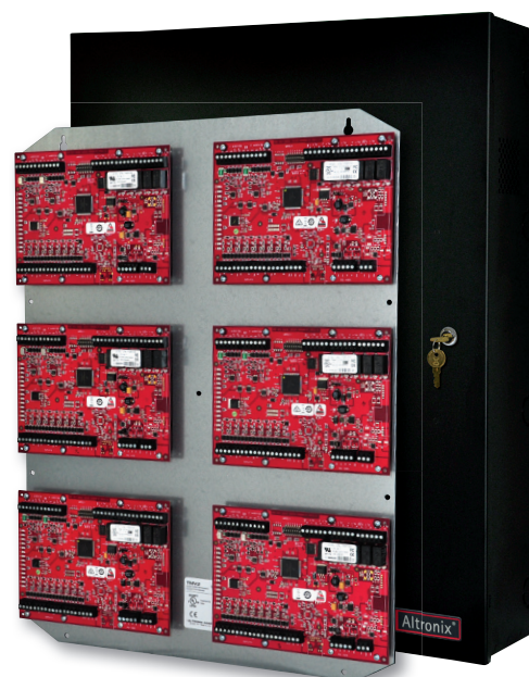
TMV2 with optional Mercury/LenelS2 boards
