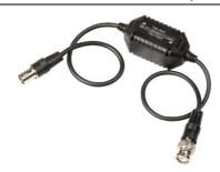
Thank you for your purchase of the **TVIGL** video ground loop isolator. This unit is designed for eliminating ground loop issues with high-definition cameras and can easily install in a new or existing system where a video signal is transmitted via one cable between two points with different ground potentials. Differences in ground potentials are typically caused by unbalanced power load lines.
