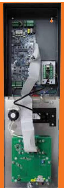
Adding a TX3-CX-1NP single door module will provide card access control.
