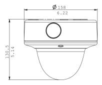
Dimensions in mm (in.) for the FlexiDome<sup>XT+</sup> impactresistant, surface mounting model
